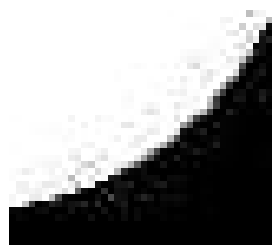
Figure 2: A low quality JPEG image showing some artifacts at the transition between black and white.
