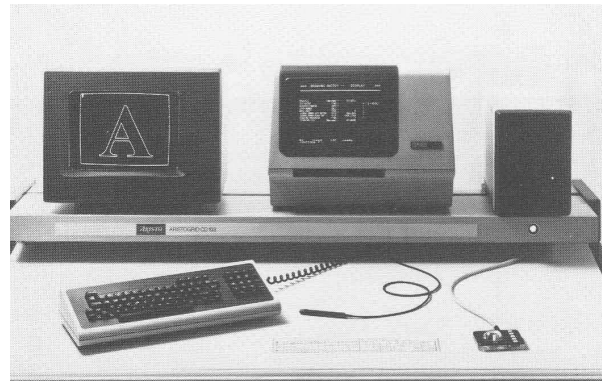
Figure 2: Typical desktop in 1972 with digitizer tablet, “mouse”, keyboard (below), direct VDT, alphanumeric terminal, electronic digitizer.
