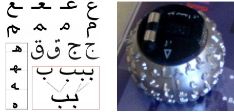
Fig. 9. The four shapes of Persian letters and their reduction to two shapes in most cases (left; uncredited Web image) and IBM's Persian golf-ball print mechanism (personal photo).
